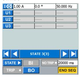
During the third step, the WIP-1 relay will start its own self-testing procedure. Several contacts will click if everything is all right, the test will end with "Press select button" and display will show "Test current Switch Off"
