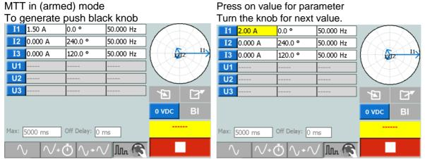
Note: When one or two phase test is made the not used phase/phases has to be set to zero.
